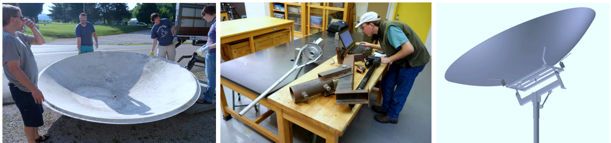
Early work on the project. Left to right: WKU physics students retrieving the 10-foot satellite dish in Summer 2016, a student studying the original mount system in Spring 2017, and a Summer 2017 engineering model of the original mount, which was unable to point at all desired celestial targets and thus required upgrading.
