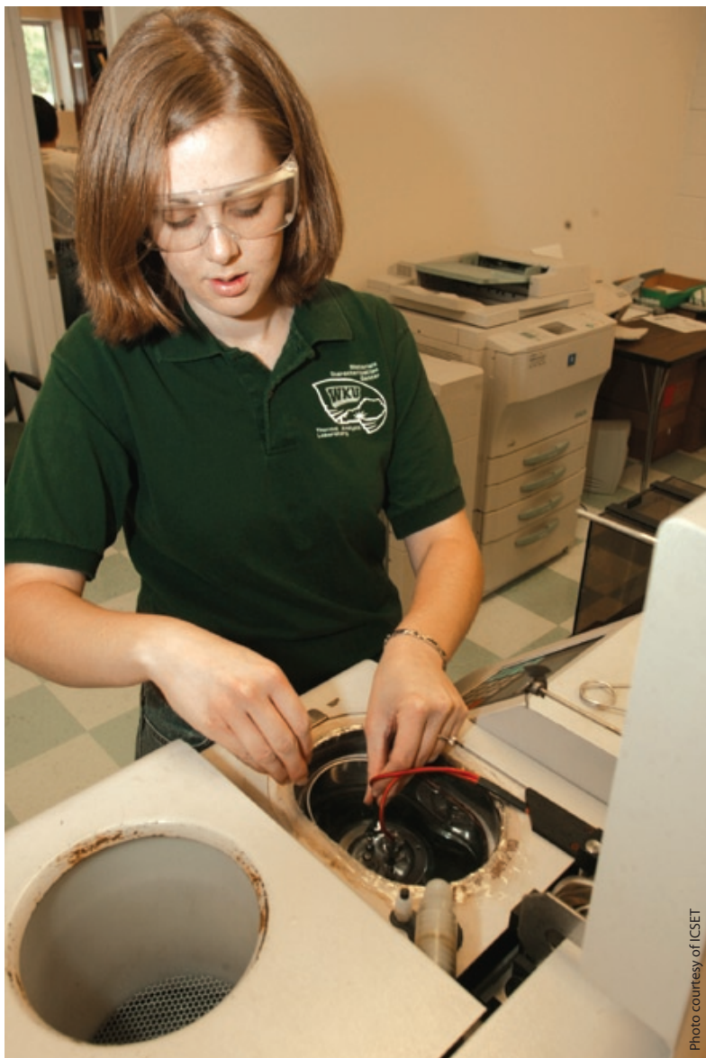
Ginger King, an undergraduate chemistry student working in Western's Institute for Combustion Science and Environmental Technology, uses a bomb calorimeter to determine the chlorine content in coal ash.
