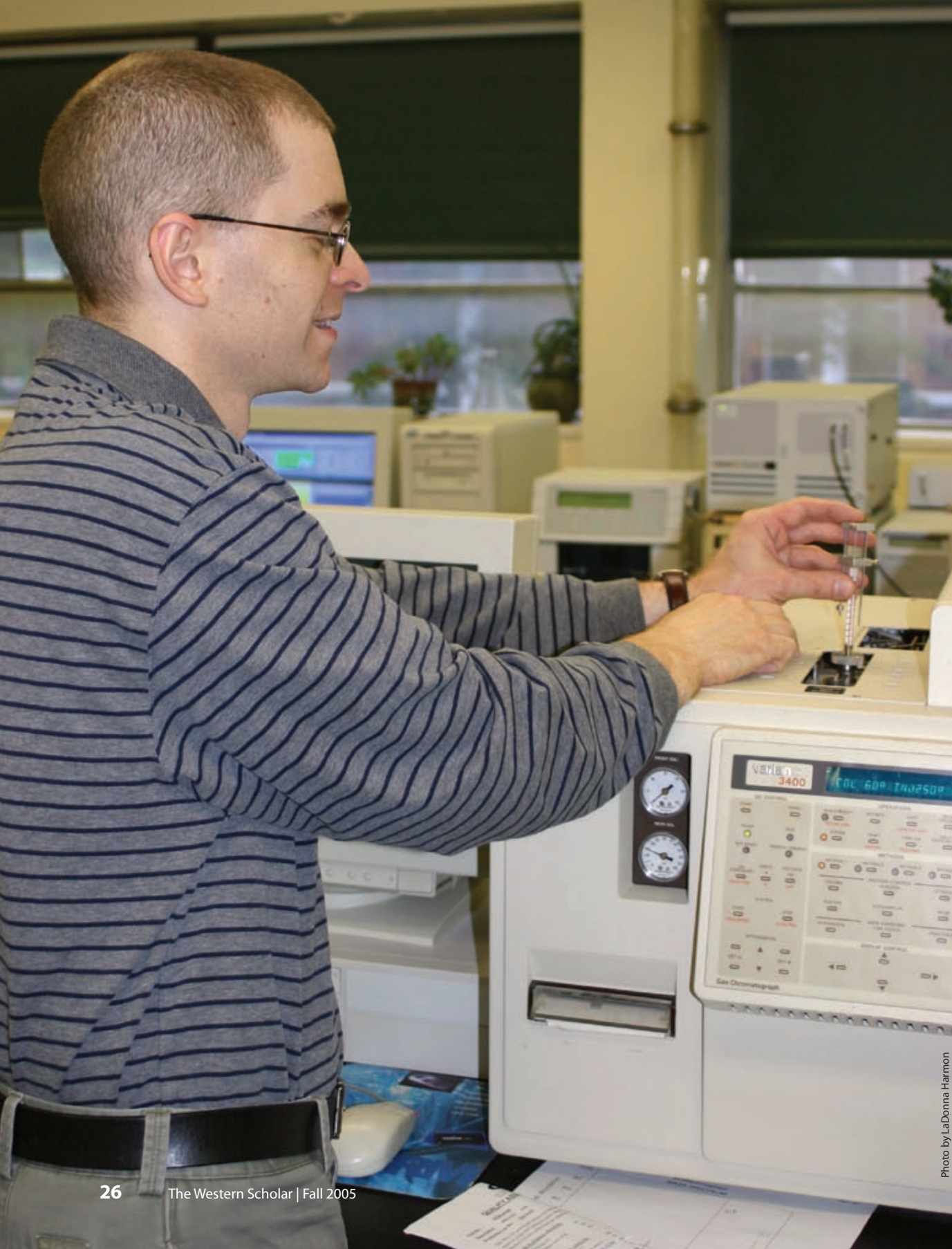
Dr. Conte injects a sample into a gas chromatograph.
