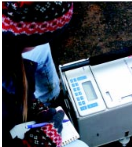
Leigh Ann Croft, a research hydrologist, takes microgravity readings using a LaCost and Romberg Microgravity Meter.
