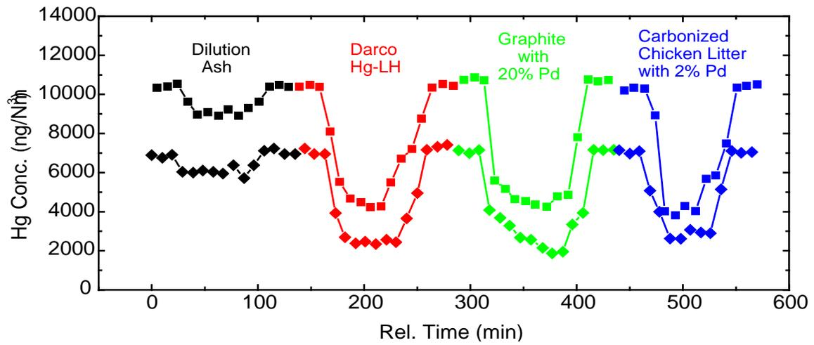
Figure 3. Onsite mercury capture data for selected samples with an adsorbent injection rate of 4 lb/MMacf (squares represent Hg(T) and diamonds represent Hg(0))
