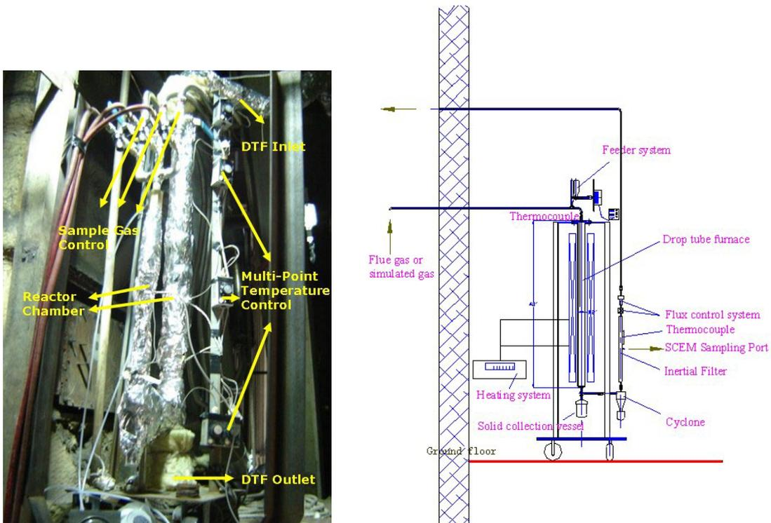
Figure 1 Drop Tube Furnace
