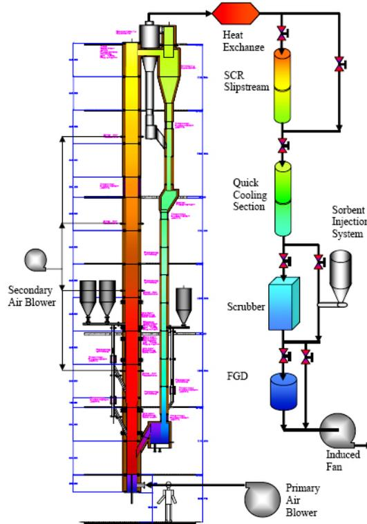
Schematic of circulating fluidized-bed combustion (CFBC) systems.
