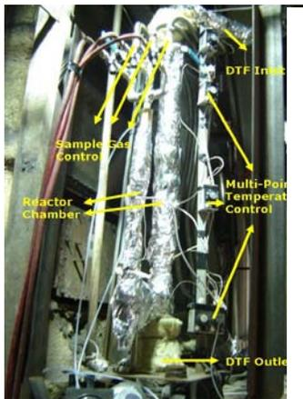
Figure 1. Drop Tube Furnace
