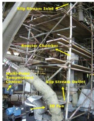
Figure 2. Entrained Reaction Facilities
