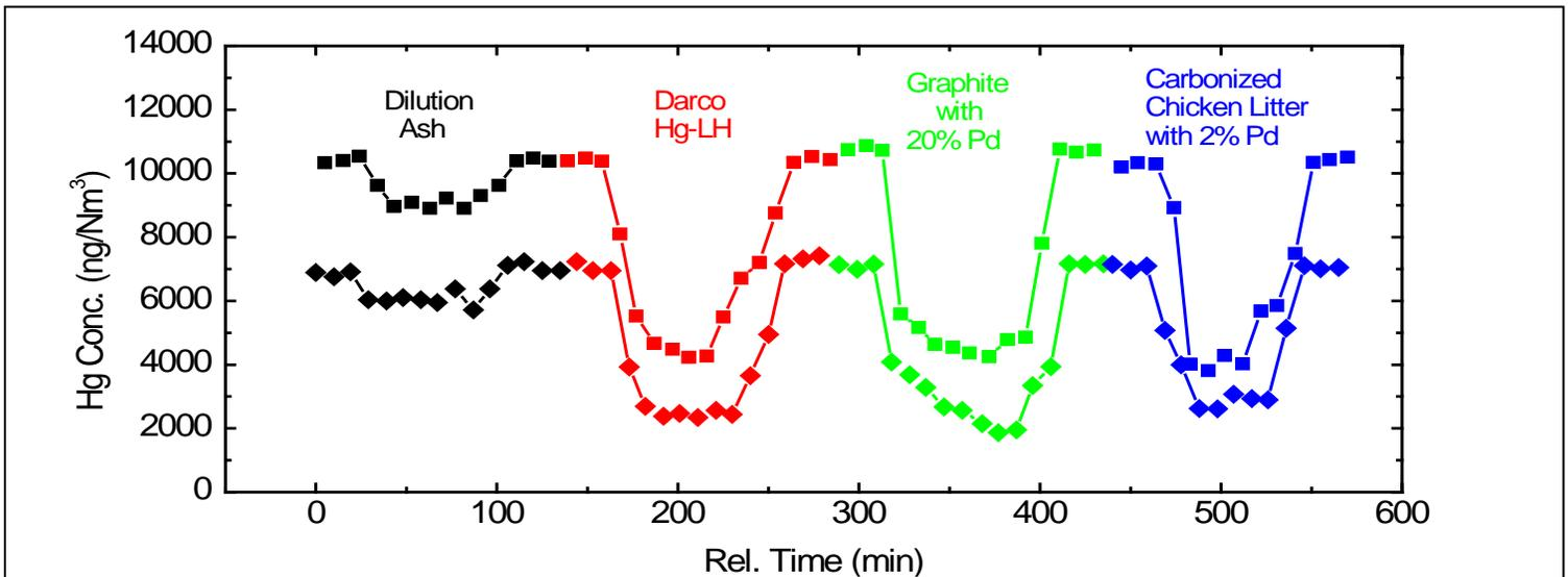
Figure 3. Onsite mercury capture data for selected samples with an adsorbent injection rate of 4 lb/MMacf (squares Hg(T); diamonds Hg(0))
