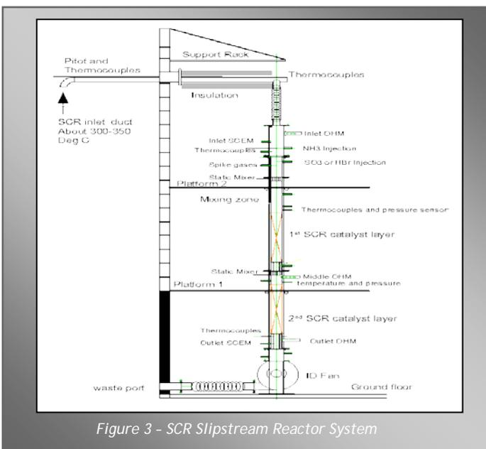
Figure 3 - SCR Slipstream Reactor System
