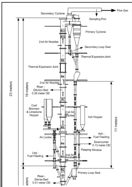
Figure 1 - 0.6 MW<sub>th</sub> CFBC System
