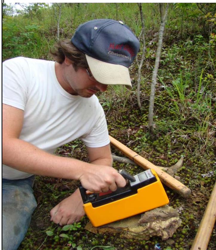
Geology student Ryan Hart taking a field measurement with the hand-held Gamma-Ray Scintillometer.
