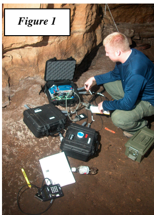
Figure 1: WKU Geology major Ben Estes examines computer data loggers that record water flow and chemical conditions every two minutes. Figure 2: Stacy Antle, research technician with the USDA ARS collects a water sample from a waterfall within the cave, using a collection device that allows him to avoid a soaking while sampling. Figure 3: Alanna Storey, a WKU undergraduate from Bowling Green, takes pH readings from the waters of Barrel Falls within Cave Spring Caverns. Photos by Chris Groves.
