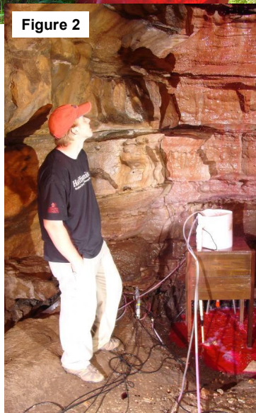
Figure 1: Brian Ham (left) and Rick Fowler (right) laying the groundwork for the epikarst dye trace study. Figure 2: Brian Ham monitoring the sampling station inside Crump's Cave. Artificial rainfall containing pink fluorescent dye penetrated the epikarst and delivered fecal pollution to Crump's Cave waterfall within two hours. Figure 3: HERI student Josh Bennett prepares some of the hundreds of samples collected during the dye trace for fecal and E. coli analysis. Other participating students are contributing field work, laboratory analyses, and computer expertise as part of the collaboration.
