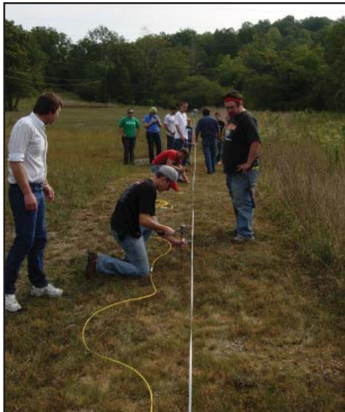
Figure 2. Wittenberg University geology students use Electrical Resistivity Ground Imaging to look for cave passages near the park.
