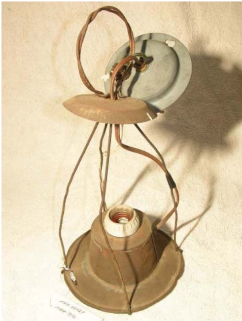
Figure 20. Likely the last production run of Mammoth Cave lanterns, many of these were wired and used to light the hotel's Woodland Cottages until they were removed in the summer of 1996. Note the beveled heat deflector.
